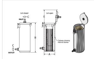
INLET/OUTLET connections available for 16mm and 20mm ID. Allow minimum clearance required for servicing as per table below (E).
